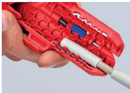
Stripping of a NYM cable
