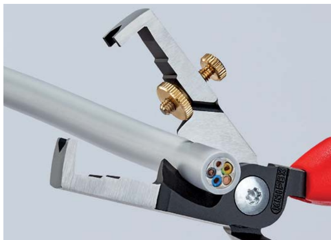
Induction hardened shear blade with precisely ground cutting edges for crushing-free cutting of copper cables up to Ø 15 mm (5 x 2.5 mm 2 )
