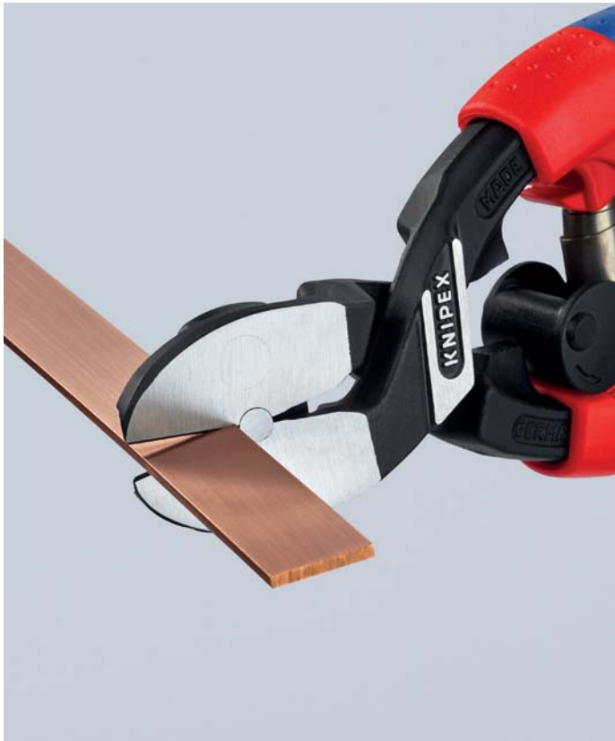
Copper busbars are cut cleanly and flush
