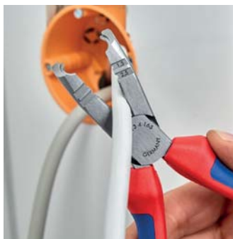
Cutting cable up to Ø 13 mm
