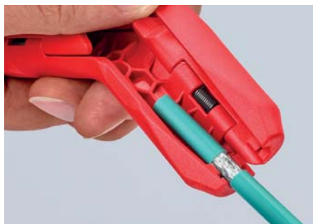
Stripping of a data cable
